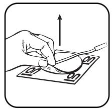
Remove an electrode by lifting its edge.
