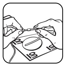
Hold the pin connector while disconnecting or inserting pin.
